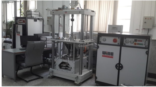
Figure 1. The multidirectional simple shear device which is used in this research.
