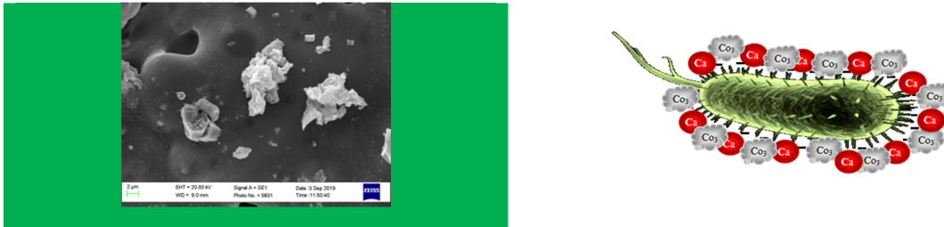
Figure 1. Left: Calcium carbonate crystals bacterially precipitated inside a LWA, Right: Schematic extracellular calcium carbonate formation.
