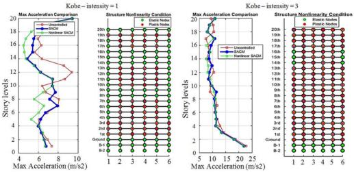
Figure 1. SACM and Nonlinear SACM results in controlling acceleration of stories and plastic hinges condition.
