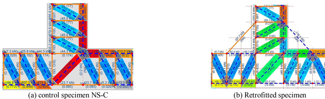
Figure 4. Detailed view of forces in critical strut-and-tie element in enlarged joint region for control and retrofitted specimens.
