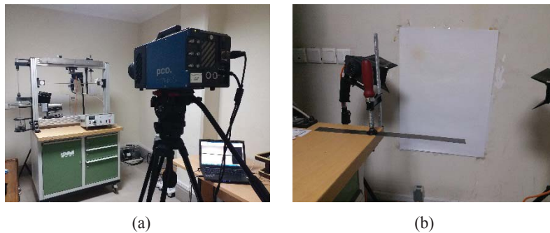
Figure 1. Camera measurement, (a) experimental setup and (b) cantilever beam.
