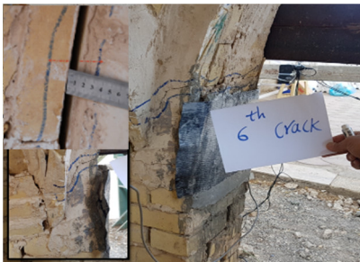
Figure 3. Separating Mortar and fiber reinforcement from bricks in the reinforced structure.
