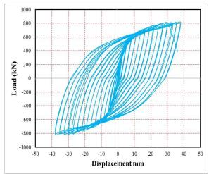
Figure 3. Shear force-displacement curve of specimen
