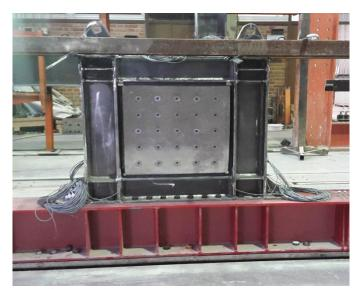
Figure 1. The one-story one-bay CSPSW specimen
