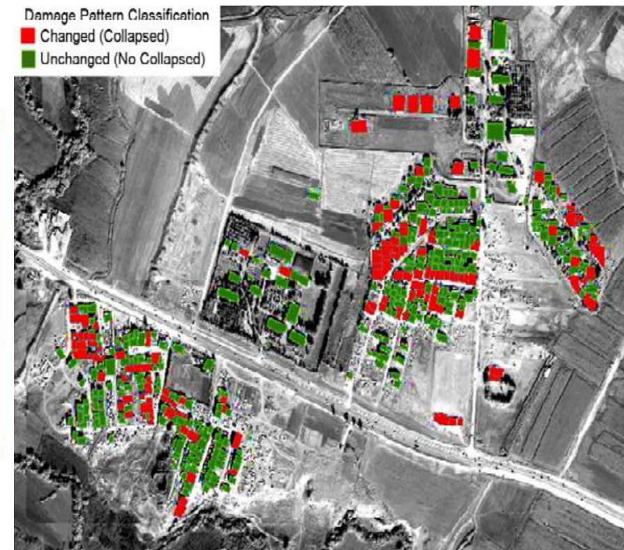
Generated Ground Truth Map by visual interpretation of post-earthquake Pleiades-1A satellite image.
