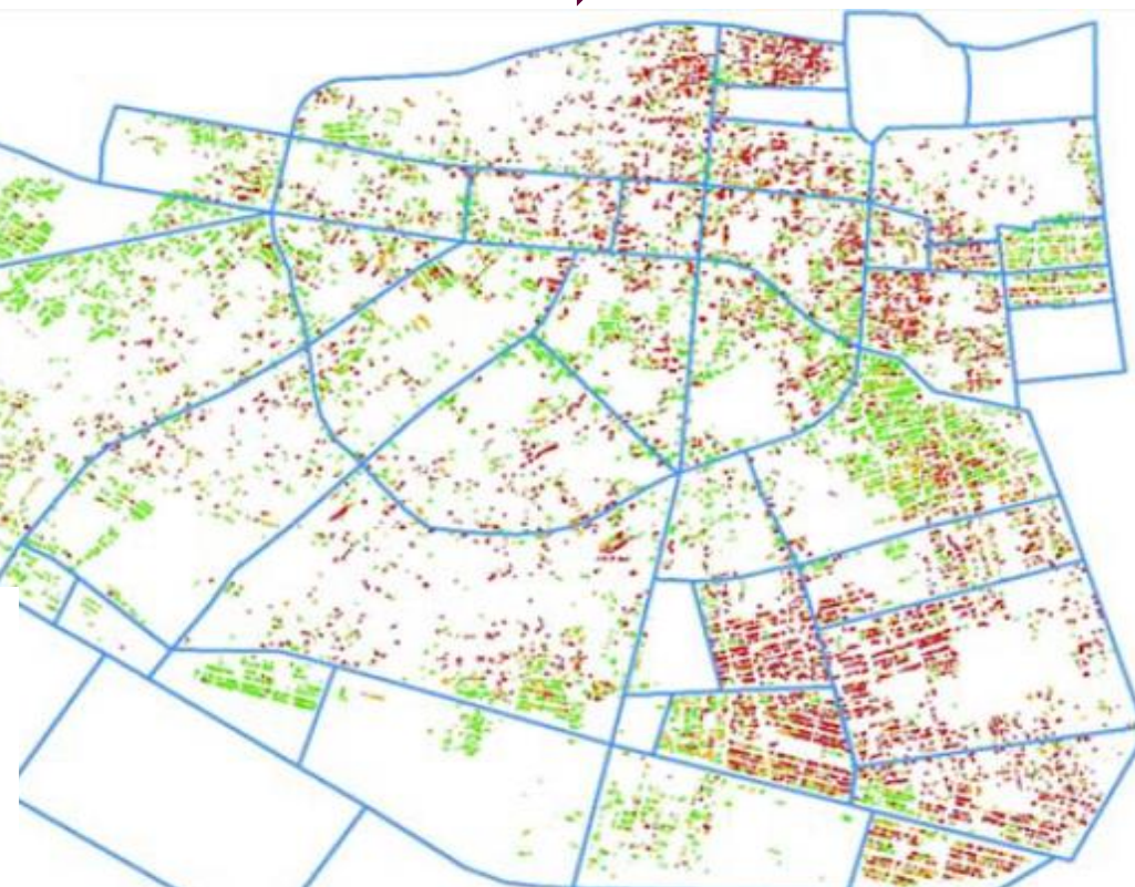
Damage mapping after BAM Earthquake - by ANN - (2015)
